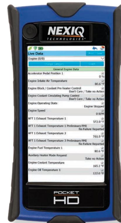
The Pocket HD handheld scan tool provides immediate access to critical diagnostic information. Pocket HD comes loaded with both Heavy Duty Standard (HDS) and Light and Medium Truck 2016 (LMT).
